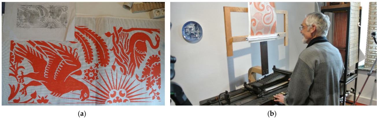
Figure 2. (a) Transfer of a pattern to squared paper, (b) Translating the design into punched cards.
