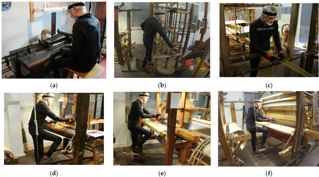
Figure 7. Examples of tasks of textile manufacturing. (a) Creation of the punch cards; (b) Wrapping of the beam; (c) Preparation of the beam; (d) Small-size loom; (e) Medium-size loom; (f) Large-size loom.
